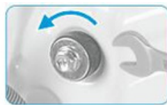
Loosen the 4 transport bolts with a spanner.
