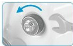
Loosen the 4 transport bolts with a spanner.
